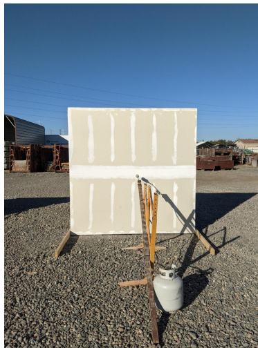
Before - Gypsum Wall 5/8" Fire Shield Type X 2x4 Wood Studs
