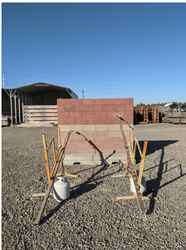
Before - Masonry Wall 6" Brick Block 8" Precision CMU 8" Shot Blast CMU
