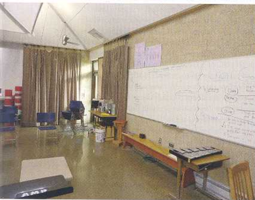
The polished concrete floor at the Da Vinci School's LEED Platinum freestanding classroom project provides thermal mass for a passive heating and cooling system. This resulted in the elimination of an HVAC system.
